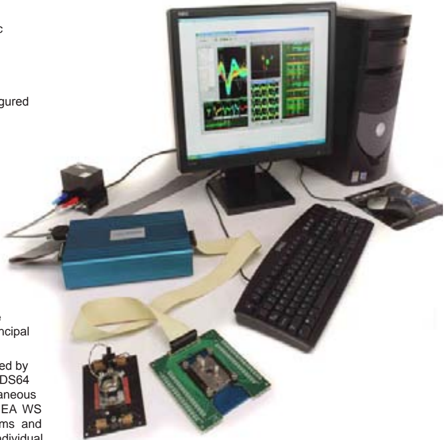
Typical MEA workstation with PC, data acquisition cards, preamp, and headstage.
